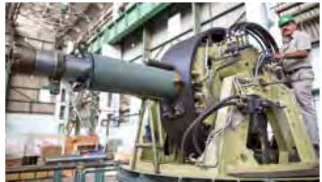
Super Rapid Gun Mount (SRGM) for Indian Naval Ships under construction at HEEP, Haridwar
